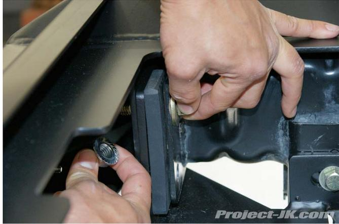
17. Using a 3/4" socket and wrench, tighten up the (4) mounting bolts and nuts on the inside of your Jeep JK Wrangler's frame rails as shown in this pic.
