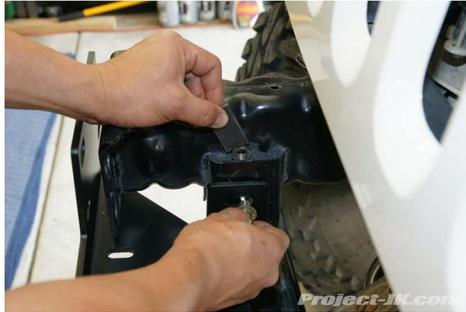
**14.** Slide one of the steel spacers in between the LoD Signature Series winch plate and frame rail bumper mount on your Jeep JK Wrangler. Then, insert the long bolts and washers provided with the bumper through the mounting holes and spacer as shown in this pic.
