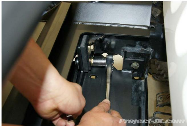
18. Accessing the bolts and nuts through the fog light holes on your LoD Signature Series JK Front Winch Bumper, tighten up the (4) mounting bolts and nuts located on the outside of your Jeep JK Wrangler's frame rails using a 3/4" socket and wrench.
