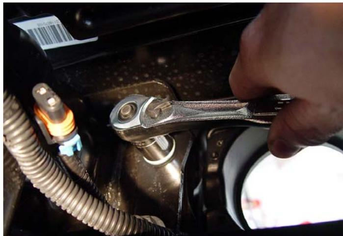
**7.** Using an 18mm socket, remove the 4 bumper mounting nuts (2 on each side) located next to the outside of your Jeep JK Wrangler's frame rails.
