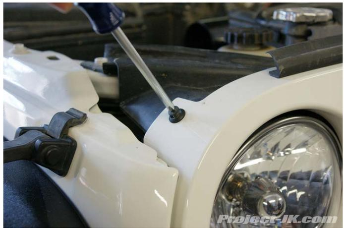
**24.** Once loose, the entire plastic screw and expansion sleeve should pull up and out of their mounting holes.
