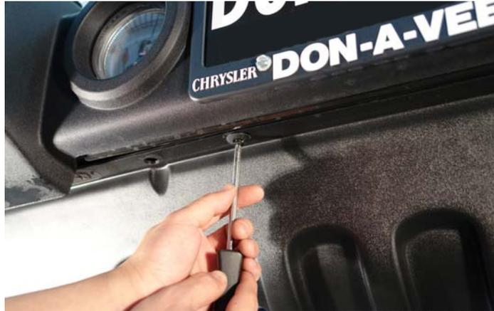
**2.** Once unscrewed, you should be able to pull out both the plastic screw and insert with little effort but if you find that your screws are just spinning (as several of mine did), you will need to wedge a flathead screwdriver or small pry bar between your JK's plastic bumper and air dam to help you force it out as shown in this photo.
