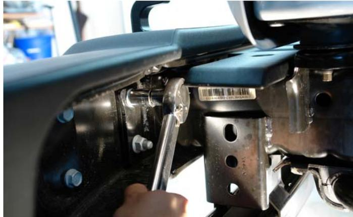
**8.** Remove the backing plates off the bumper mounting studs as shown in this photo.
