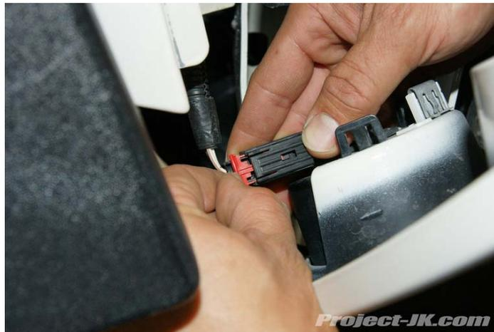
**26.** Squeeze the wiring harness plug and pull it out of your Jeep JK Wrangler's indicator light socket. You can now pull the grille off and set it aside for now.
