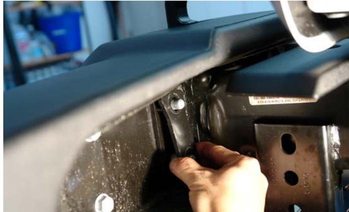
**9.** Carefully pull off your Jeep JK Wrangler's front bumper off the frame rails. If your JK came equipped with factory tow hooks, grab and use both of them to carefully pull your front bumper off the frame rails.
