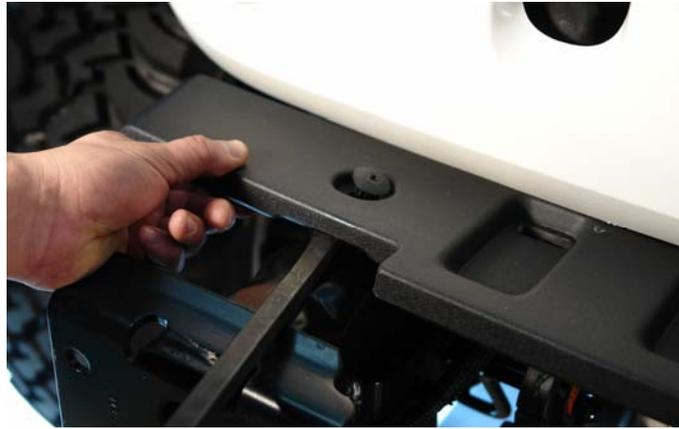
**12.** Again, if your Jeep JK Wrangler came equipped with factory fog lights, use a phillips screwdriver to remove the 4 screws securing them to the bumper. Then, pull the fog lights out and set them aside until you are ready to install them in your new LoD Signature Series JK Front Winch Bumper.
