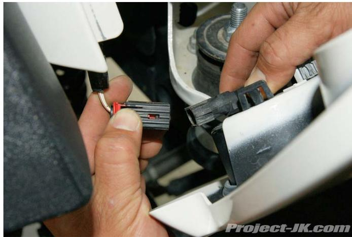
**27.** At this point you will need to extend your factory wiring harness to the fog lights since the fog lights are now relocated to a wider position than before. After lengthening the wiring plug your Jeep JK Wrangler's factory wiring harness back into the fog lights.
