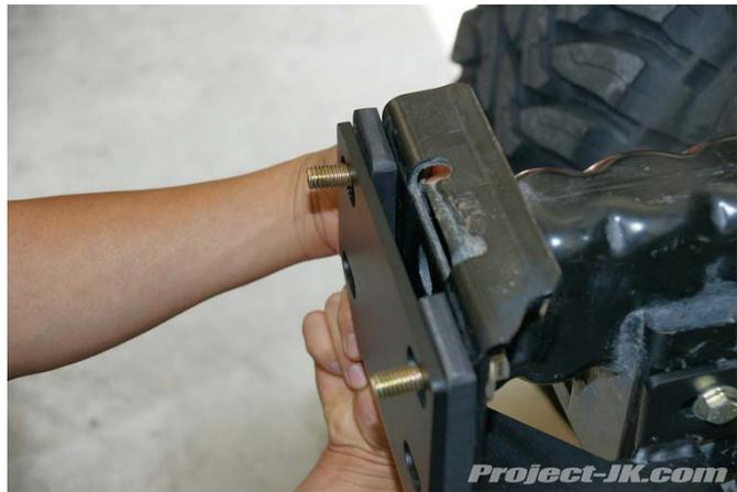
16. With the help of a friend, carefully place your new LoD Signature Series JK Front Winch Bumper on to the frame rails of your Jeep JK Wrangler and slide the mounting holes through the bolts you just installed. Reaching from the back, loosely secure it in place using the nuts provided.
