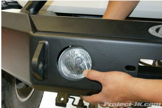
**22.** Secure your Jeep JK Wrangler factory fog lights on to your LoD Signature Series JK Front Winch Bumper using the nuts provided. You will need a 3/8" socket for this job.
