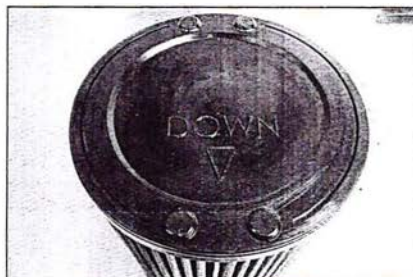
6. Notice that the Windstorm Filter top has a directional arrow in the center and locating lugs in the 12:00 and 6:00 positions.
