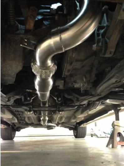
9. Make sure all connections are completely seated and tighten clamps at the actual connection points (on the areas where the pipe is relief cut. There should be no overlap of pipe.
