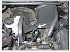
17. Secure the transmission vent hose to the heat shield with the provided tie wrap passing through the hole in the bottom of the heat shield.
