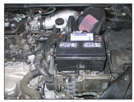
23. Reinstall and secure the battery, reconnect the positive battery cable.
