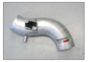
14. Install the mass air sensor into the K&N<sup>®</sup> intake tube and secure with the provided hardware.
