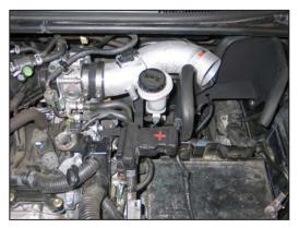
20. Install the K&N<sup>®</sup> intake tube into the silicone hose on the throttle body and align with the mounting bracket installed in step #19. Secure with the provided hardware and hose clamp.
