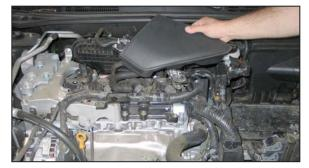
2. Remove the two retaining clips which secure the fresh air supply duct to the core support.
