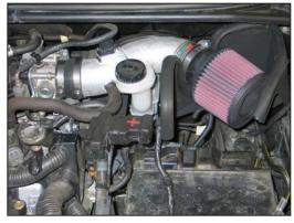
22. Install the K&N<sup>®</sup> air filter onto the K&N<sup>®</sup> intake tube and secure with the provided hose clamp.
