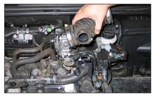
9. Loosen the hose clamps which secure the intake tube and then remove the intake tube from the vehicle.
