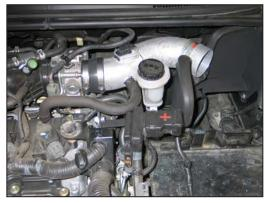
21. Install the crankcase vent hose onto the K&N<sup>®</sup> intake tube and secure with the factory hose clamp.
