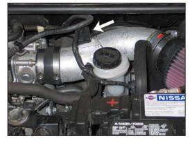
25. Reconnect the mass air sensor electrical connection.
