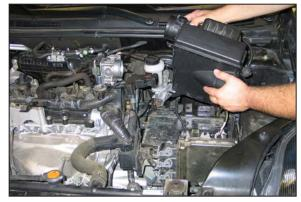
12. Remove the airbox from the vehicle. NOTE: Be patient while removing the airbox, it is a tight fit and requires some maneuvering to get out. Loosening the battery tray bolts will ease removal but is not absolutely necessary. On automatic equipped vehicles, be sure to reattach the battery tray and TCM module. NOTE: K&N Engineering, Inc., recommends that customers do not discard factory air intake.
