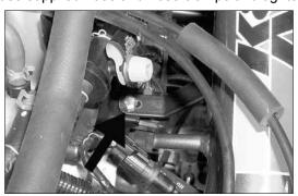
19. Secure the bracket to the original mounting point using the provided hex bolt and wave washer as shown.
