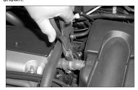
3. Depress and slide the hose clamp off the crank case vent connection at the air cleaner assembly as shown.
