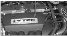
25. Reinstall the engine cover and secure with the original hex bolts as shown.
