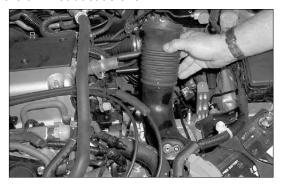
11. Remove the air inlet duct as shown.
