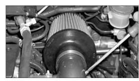
23. Install the K&N® air filter onto the K&N® intake tube, then, secure with the provided hose clamp as shown.
