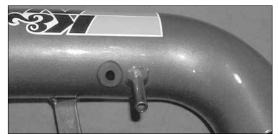
16. Install the provided grommet into the hole on the  $K\&N^{@}$  intake tube as shown.
