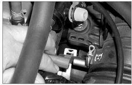
5. Disconnect the IA bypass control thermal valve vent hose from the stock intake tube as shown.
