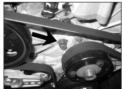
10. Remove the front engine bolt shown.
