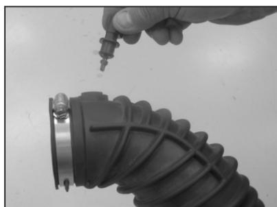
7. Remove the air temperature sensor from the stock intake tube as shown.
