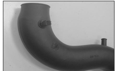
8. Install the air temperature sensor into the grommet installed into the intake tube during step #6.
