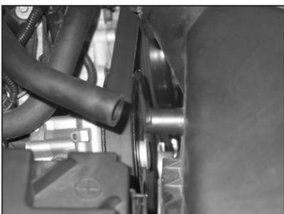
3. Disconnect the crankcase vent hose from the stock intake tube as shown.
