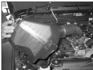
5. Lift up the airbox assembly to dislodge it from the mounting grommets and then remove the complete assembly from the vehicle.
