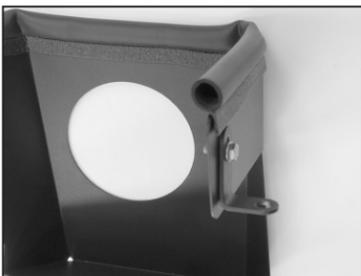
17. Install the supplied "L" bracket (070712) onto the heat shield as shown with the provided hardware.
