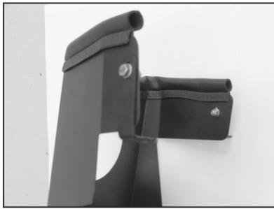
18. Install the supplied "L" bracket (07195) onto the heat shield as shown with the provided hardware.
