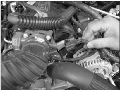
2. Release the locking tab on the air temperature sensor electrical connector and then disconnect the connection.
