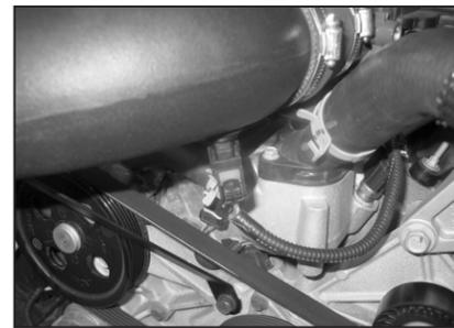
25. Reconnect the air temperature sensor electrical connection.
