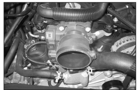
9. Install the supplied silicone hose onto the throttle body and secure with the supplied hose clamp.
