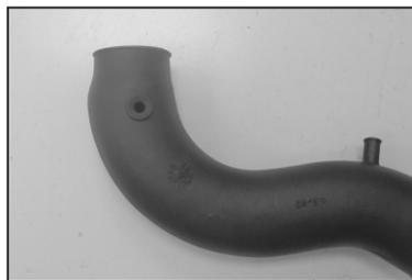
6. Install the supplied grommet into the hole in the intake tube as shown.
