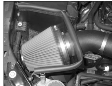
24. Install the K&N® air filter assembly on the intake tube and secure with the provided hose clamp as shown.
