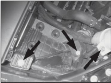
13. Remove the power steering reservoir mounting bolt and the two airbox bracket mounting bolts shown.
