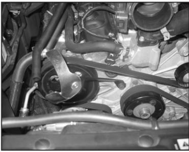
12. Install the tube mounting bracket assembly onto the engine and secure with the bolt removed in step #10.
