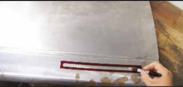
**4.** Next, cut along the lines marked out for the light strip using a cutoff wheel.
