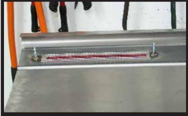
Attach the red Lexan insert to the clear diffueser and line up in the cut hole.
