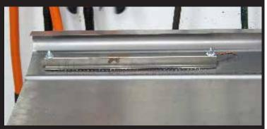
**9.** Attach the U-shaped bracket, with the LED bar, to the back of the panel and secure with lock washers and nuts.
