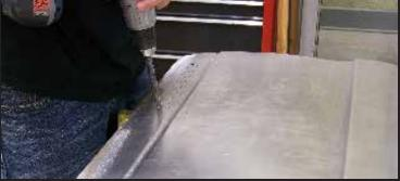
**3.** To keep the corner ends round, drill a ½-inch hole on each end of the light cutout.
