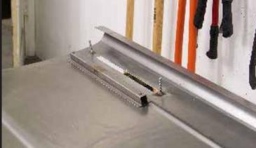
Weld two bolts to the inside of the combo skin that lines up with the holes in the U-bracket.
