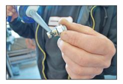
**Step 5** - We recommend applying a small amount of silicone to the splined area of the Grip-Sert.
