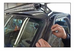
**STEP 14** - Route the power wire down the A-pillar under door seal and wire the light bar as noted in the light bar instructions.
