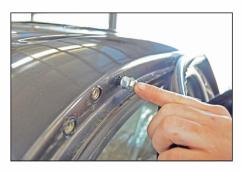
**Step 6** - Insert supplied Grip-Sert rivet nut into holes flush with the metal surface.
