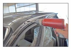
**Step 4** - Drill marked holes with a 5/64" pilot drill bit and then slowly step up to a 3/8" drill bit.
