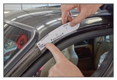
**Step 2** - Place the template in the base of the rain gutter, lining up the A-pillar and roof seam marks.
