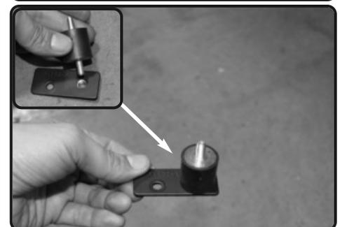
11. Now install the M6 vibramount to the threaded fitting on the provided bracket. Secure and tighten.
