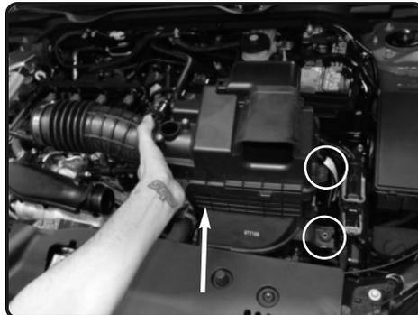
5. Loosen the 2 bolts holding in the air box and remove. Lift up and remove the complete stock air box assembly out of vehicle.
