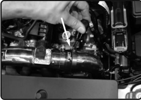
**24.** Install the 2-3/4" straight hose with clamps to the upper intake assembly
