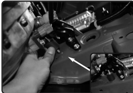
**21.** Install the vibramount to the three-threaded insert on frame. Secure and tighten.
