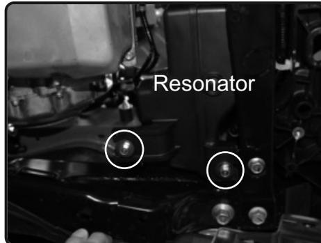
6. **Now with vehicle on a lift or on jackstands secured, remove front bumper cover.** From under the vehicle, pull back splash guard, loosen the 2 bolts holding in the resonator box.
