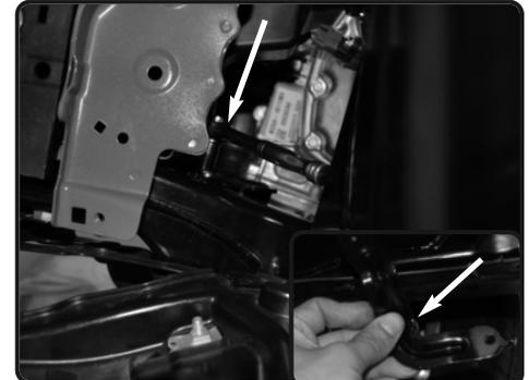
7. Loosen the 1 screw holding in the resonator bracket. Remove the bracket from the vehicle.
