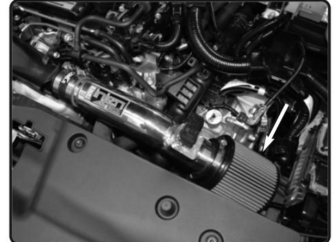
**19.** *For extreme weather conditions, install filter on upper intake tube assembly for Short Ram Application.*
