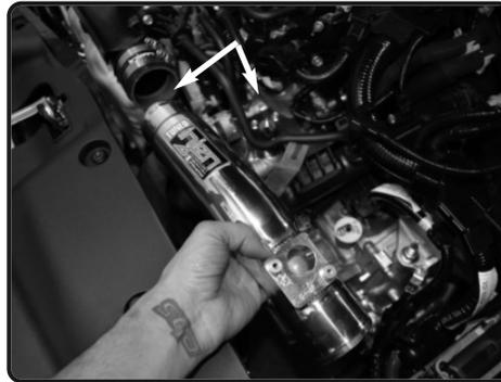
**14.** Install the upper intake tube assembly into vehicle and position tube to straight hose and bracket to vibramount.
