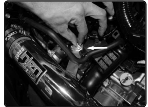
**15.** Secure the upper intake tube assembly bracket using M6 nut and fender washer.
