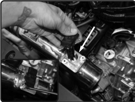
**16.** Install the MAF sensor into the machined pad. Secure using 2 screws from step 4.
