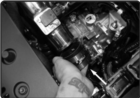
**20.** Install the 2-3/4" straight hose with three clamps to the upper intake assembly
