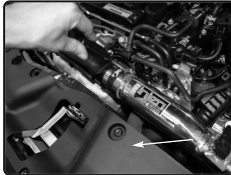
**18.** Tighten the clamp on straight hose.
