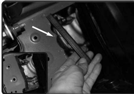
**22.** With provided rubber trim, install to the edge of frame. This will prevent any contact with intake tube and frame.
