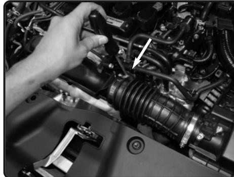
7. Loosen the clamp on the turbo housing using phillips screwdriver.
