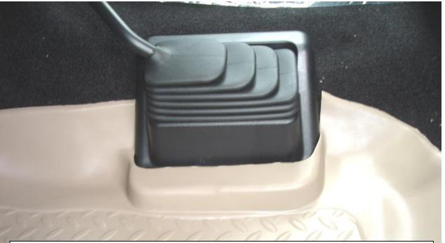
PART #3386 SHOWN TRIMMED FOR A MANUAL TRANSFER CASE SHIFTER. TO TRIM, SIMPLY REMOVE THE LOWERED SECTION ON THE LINER.
