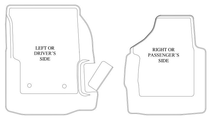
IF YOUR SUPER DUTY TRUCK IS EQUIPPED WITH A MANUAL TRANSFER CASE SHIFTER, YOU WILL NEED TO TRIM YOUR LINER AS TO ALLOW IT TO FIT AROUND THE SHIFTER. TO TRIM, REMOVE THE MATERIAL FROM THE LOWERED AREA ON YOUR LINER AS DEMONSTRATED ABOVE. USE THE EDGE OF THE LOWERED AREA AS YOUR GUIDE. A PHOTO OF THE TRIMMED LINER IS SHOWN ON THE BACK OF THIS PAGE. A UTILITY KNIFE OR HEAVY SHEARS WORK WELL FOR TRIMMING.
