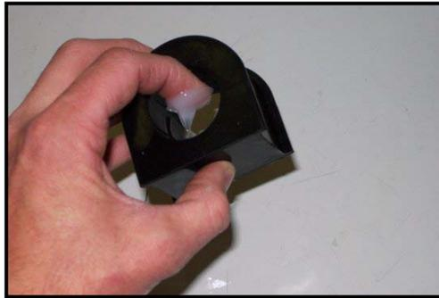
8. Install the urethane bushings on the bar. Make sure you position the bushing so when the bar is installed in the vehicle, the split will face the front of the car.
