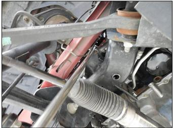
Figure 1 - Access to top bolts passenger's side
