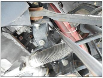
Figure 2 - Access to top bolts driver's side
