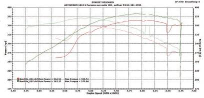
After the I-M Shield was installed, the LS1 cranked out 382 horsepower and 370 lb-ft of torque. That's a gain of 18 and 20, respectively.
