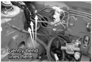
7 Next flip the bracket on the prop valve so it can be used to mount it to the firewall. You'll need these tools; C-clamp with a 4" opening and T-30 Torx Security Bit. Use the C-clamp to hold the prop valve together and unscrew the two T-30 Torx screws holding the bracket on. Flip the bracket towards the firewall as shown in the picture and retighten the screws.
