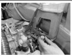
Now that the engine is supported by the left and right-hand mounts we can connect the rear mount to the chassis bracket and transmission bracket. Using the two M12 x 60mm bolts with washers and nuts bolt the rear mount int both the rear chassis bracket and rear engine bracket.
