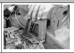
4 Using the M12 x 35mm bolt and two M12 x 30mm bolts with washers, bolt the Hasport mount and bracket to the transmission. Leave the bolts finger tight at this time.
