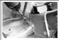
A chisel and hammer can now be used to finish removing the bracket. Once it is off use the die grinder with a sanding wheel to remove any left over material.
