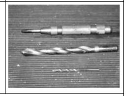
Begin by center punching all the spot-welds on the mount. This is so the drill bit won't drift when drilling.
