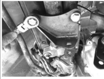
Finally, using the two M12 x 60mm bolts provided by Hasport install the new rear engine bracket. Use the stock bolt for the forward most bolt hole that passes through the bracket, the block, and threads into the transmission. Insert all three bolts and finger tighten. Once all three are in, tighten the bolts to 43 ft/lbs of torque.
