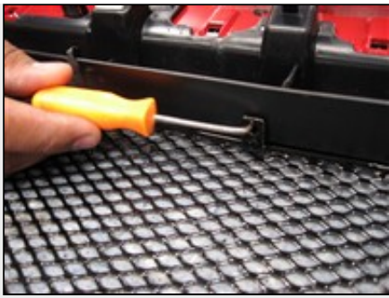
Picture #25: Mark grille mounting tab center hole locations using a sharp scribe.
