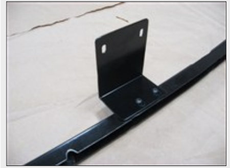
Picture #18: The new latch bracket mounted to the grille shell support.
