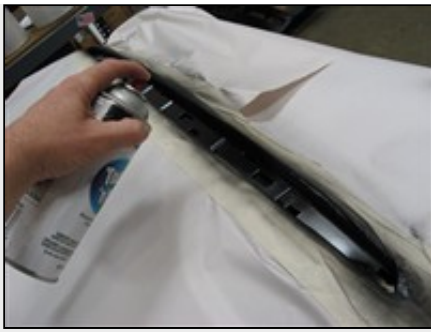
Picture #37: Tape off and paint the top grille background area using "Flat-Black" spray paint.
