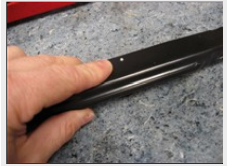
Picture #30: The metal support brace showing the area that needs a clearance hole.
