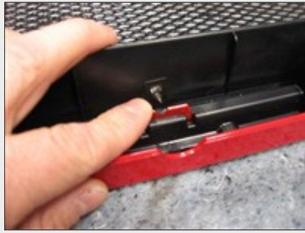
Picture #29: The lower screw tip will come into contact with the metal support brace removed earlier. We will need to make a clearance for the screw tip into the metal support.
