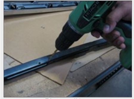
Picture #15: Drill holes for the latch bracket using 13/64 drill bit.
