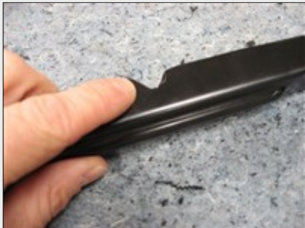
Picture #31: Using a file or drill make a notch into the support bar as shown.
