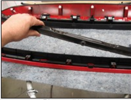
Picture #13: Remove the grille shell metal support along the bottom of the grille shell.
