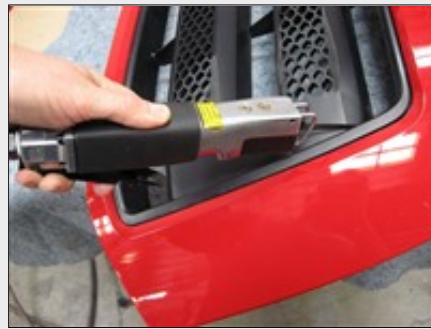
Picture #20: Cut the factory grille center bars off.
