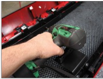
Picture #26: Drill 3/16 inch holes for Grille mounting screws.
