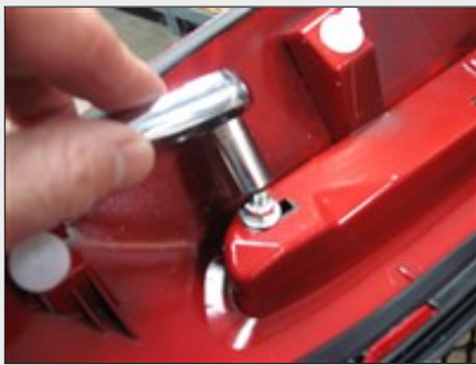
Picture #40: From the back side of the grille shell fasten top grille insert nuts.
