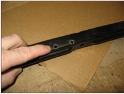
Picture #16: A view of the holes drilled into grille shell support.
