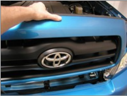
Picture #4: Pull up on the grille to remove.
