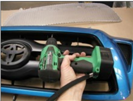
Picture #7: Drill top mounting screw holes using 3/16 drill bit.
