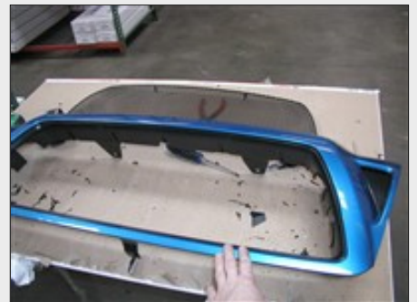
Picture #12: Optional A look at the grille shell with the center removed.
