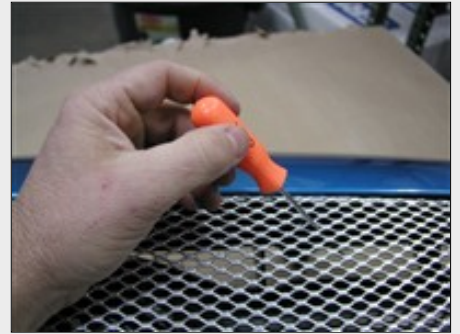
Picture #6: Place sport grille into opening while holding in place mark the top mounting tab hole location.
