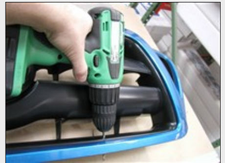
Picture #9: Drill lower mounting screw holes then fasten grille to the grille shell.
