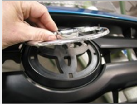
Picture #5: Unclip Toyota emblem from the back side.
