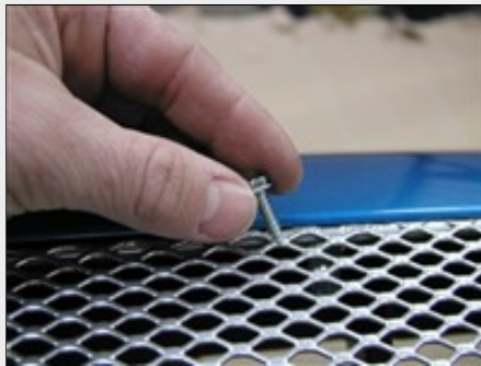
Picture #8: Place upper mounting screws in place first then mark lower mounting screw location.
