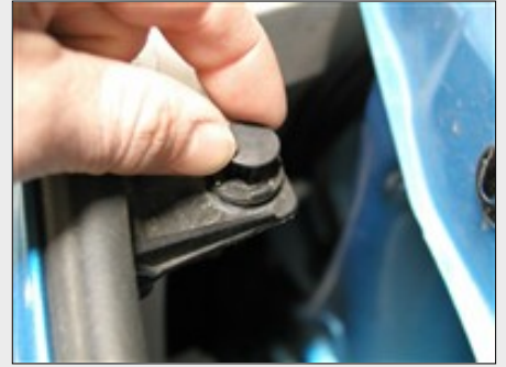
Picture #3: Remove push clips on the top of the grille shell.
