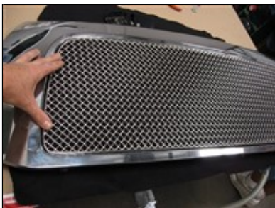
Picture #28: Place GrillCraft grille into grille shell opening.
