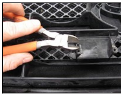
Picture #17: Remove the two plastic nubs using wire cutters.
