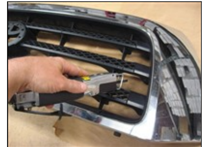
Picture #21: Cut the factory grille center bars off.
