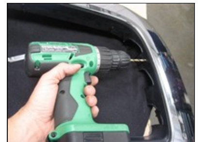
Picture #30: Drill 3/16 inch holes for Grille mounting screws.
