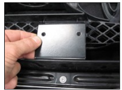
Picture #18: Place latch extension bracket onto grille as shown.
