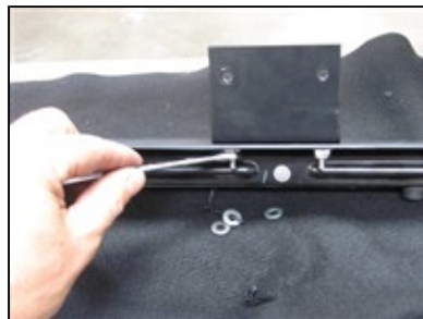
Picture #26: Fasten extension bracket with supplied hardware.
