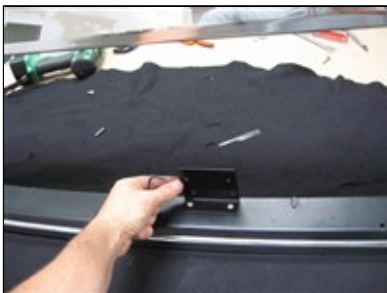
Picture #25: Mount extension bracket to grille shell.
