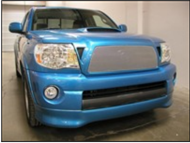
Picture #19: Shown here in silver color without cutting the grille shell center.
