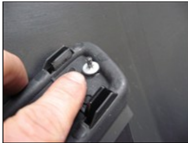
Picture #26: A view of the fastener installed.
