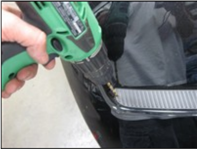
Picture #22: Drill holes for vent grille mounting pins.
