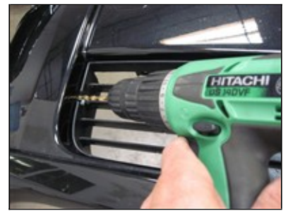
Picture #18: Drill 3/16" holes for grille mounting screws.
