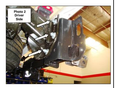
**Step-**9 With assistance attach the bumper shell brackets to each frame bracket using (2)  $\frac{1}{2}$ " x 1  $\frac{1}{2}$ " hex bolts, (4)  $\frac{1}{2}$ " flat washers, (2)  $\frac{1}{2}$ " lock washers and (2)  $\frac{1}{2}$ " Hex nuts, (Photo 3 & 4).
