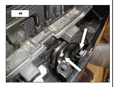
**Step-7** position the driver side upper bracket behind the bumper, align the bracket with the hole in the bumper and bumper frame bracket then reinstall and tighten the bolts, **(Photo 9 & 10)**. Repeat the above steps to install the passenger side upper bracket then reinstall the vehicle's grille, radiator cover.
