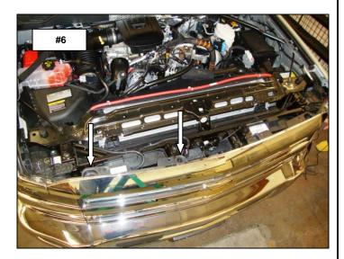
Step-5 Working from one side gently pull outward to unsnap the clips and remove the grille, (Photo 7).
