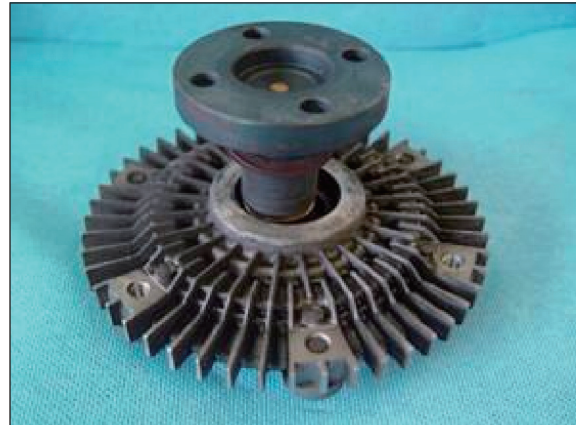
Fan clutch bearing blocked → breakage
