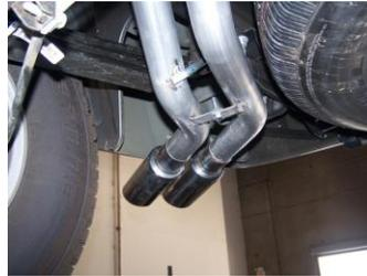
6. Now install driver side tailpipe #D. The spare tire may need to be loosened and pushed to the driver side to allow for clearance. Use bolt kit #H to attach both tailpipes together.
