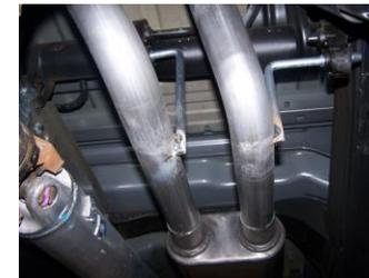
7. Using clamps #G secure both tailpipes to the outlets of the muffer. Rotate tailpipes to best fit your truck.
