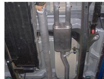
4. Install muffer #B with inlet towards Y-pipe. Use jack stands to support the muffer. Use clamp #F to secure the muffer to headpipe. Do not tighten.
