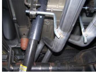
5. Make sure muffer outlets are level before installing tailpipes. Now install passenger tailpipe #C. Insert welded hangers into rubber grommets.
