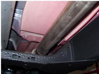
3. Bolt headpipe #A to the stock flange re-using the factory nuts and bolts. Insert welded hanger into rubber grommet. Do not tighten.
