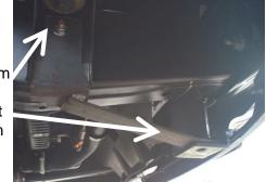
**Step 6:** When Grille is aligned, attach bottom foot of Grille to the pre-punched holes of the brackets installed in step 5. Tighten all bolts. Reattach rubber flap for proper air flow to condenser.
