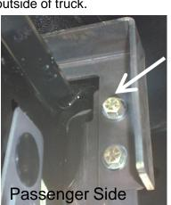
**Step 3:** (EDDIE BAUER EDITION ONLY: Remove lower bumper grille so that upper bracket can stick through bumper! Grille can be cut and reattached after install depending on customer). Attach upper support bracket to the side of frame horn bracket that was bolted on in step 2 using supplied bolts. The angle in the bracket should face the inner side of truck.
