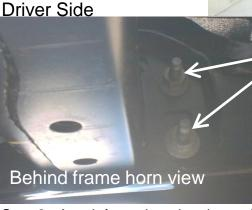
**Step 1:** Pull out plastic pegs that hold rubber flap on the bottom, but <u>do not remove rubber</u>. Remove nuts from factory bolts which are located on the inner frame horn plate as shown (2 on driver side + 2 on passenger side).
