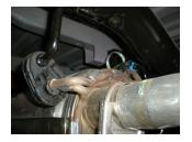
3) Support the muffler with a stand and remove the two hangers at the rear of the muffler along with the hangers in front of the muffler from the rubber mounts on the vehicle. Then remove the clamp on the slip connection just behind the catalytic converter. After removing the clamp, this connection will need to be either sliced or heated in order to separate the connection. Remove the muffler and set aside.
