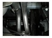
8) Install a provided 2½" clamp onto the right muffler outlet. Place the right side tailpipe **#16415S** into position over the axle and slip into the right side muffler outlet, while at the same time, connecting the hangers at the front and rear of the pipe to the rubber mounts on the vehicle. Tighten the clamp enough to hold, but still allow for adjustment.
