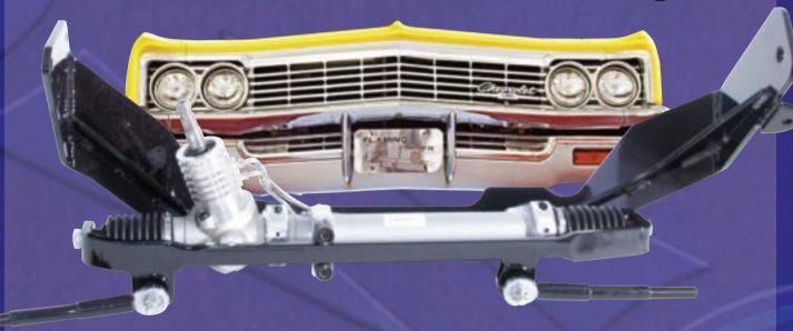
The new Flaming River 1965-69 Impala/Caprice Power Rack and Pinion Cradle Kit has over 6" of travel, provides full lock-to-lock turning radius, and has an adjustable pinion angle. This kit uses a travel bar design to properly position the steering pivot points to the original location and deliver the original turning radius. The travel bar system features a stabilizer guide clamp that provides added stability while driving. Our Rack
