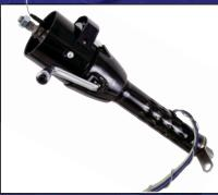
Collapsible Micro Column Shift Tilt Column p. 59
