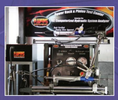
Every rack and pinion built at Flaming River is pressure and fluid tested.
