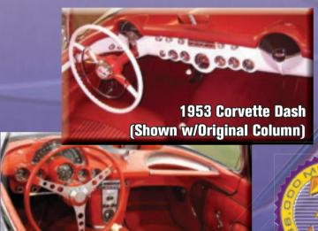
The Corvette dash was completely redesigned in 1958 with the instrument panel directly in front of the driver.
