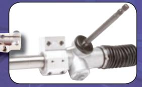
05-14 Mustang Shaft FR1515P-SHFT Provides Additional Header Clearance
