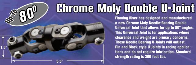
Flaming River has designed and manufactured a new Chrome Moly Needle-Bearing Double Universal Joint that allows for up to 80° angles. This Universal Joint is for applications where clearance and weight are primary concerns. These Needle Bearing U-Joints will outlast Pin and Block style U-Joints in racing applications and do not require lubrication. Standard strength rating is 300 foot Lbs.
