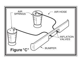
Select one air helper spring from your kit. Install the upper bracket by aligning the three holes on the air spring with the holes on the upper bracket. Fasten the upper bracket to the air spring using the 3/8" x
