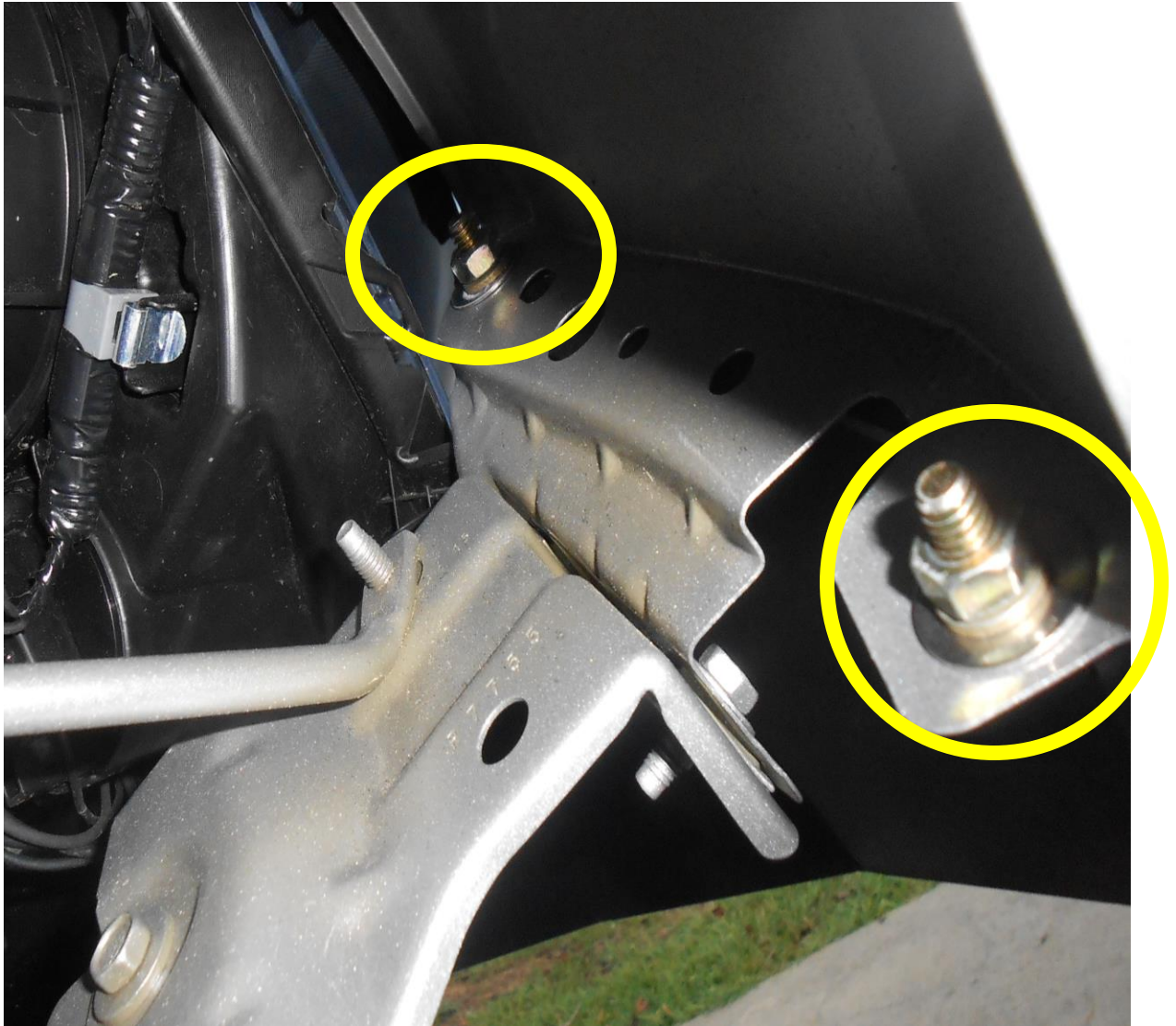
Figure 6b (bolts through mount points on fender)
