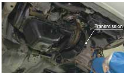
⑩ Reinstalling the Transmission
