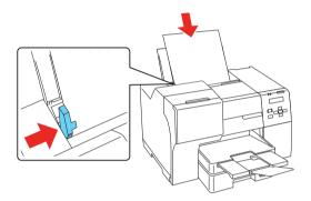
**Note:** You can load up to 150 sheets of plain, letter-size paper in the rear sheet feeder. Do not load paper above the arrow on the edge guide.
