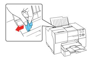
**3** Insert paper with the printable side up, against the right side of the feeder. Then slide the edge guide against the paper.
