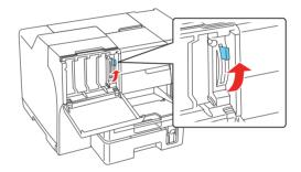
The arrow mark should be on top and pointing toward the printer.
