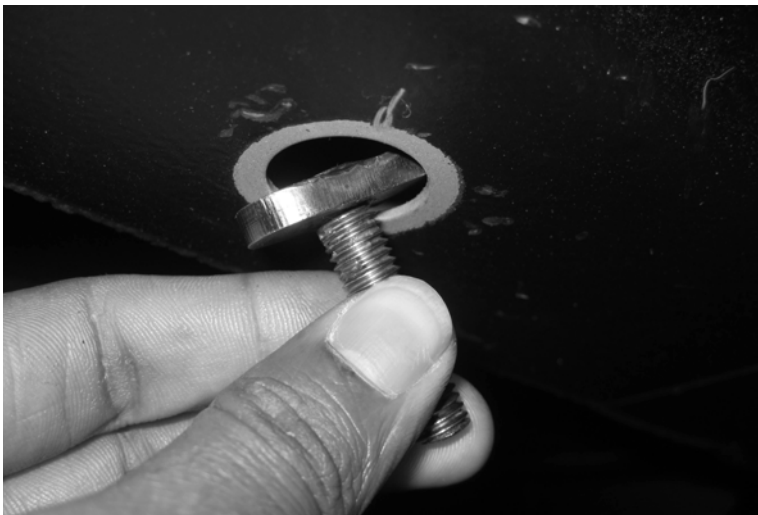
Install the M10 x 60 T-bolt
