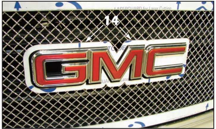
14. For customers requesting emblem reinstallation: Align the emblem surround around the factory emblem, making sure it is even and level. You might have to trim a mesh wire or two to centered it properly (mesh grille shown, E-Power similar).
