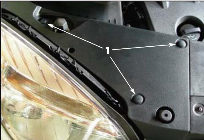
1. Open the hood and remove the six (6) plastic push fasteners (three each side) that secure the side plastic panels to the header panel, then rotate them back out of the way. Lift up on the centers of the plastic push pins using a small flat blade screwdriver to release them.
