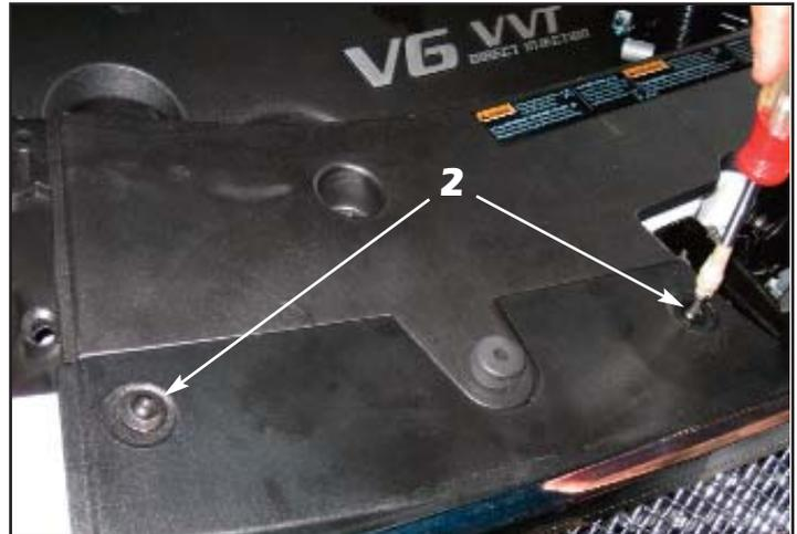
2. Use a Torx T-20 tool to remove the four (4) torx screws (2 each side) securing the top edge of the bumper cover/grille assembly to the header panel.
