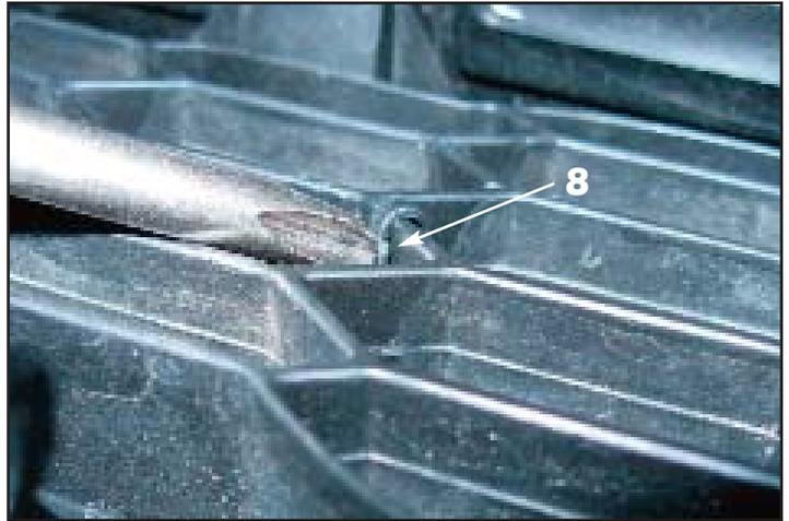
8. Use a small block of wood to press the retaining pins firmly against the mesh and bend the pins over around the factory grille to secure the pro-formed mesh grille.
