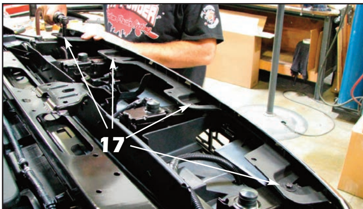
17. Reinstall the factory hardware across the top of the grille and the radiator support panel cover to finish.
