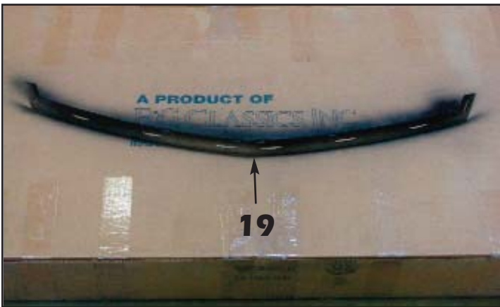
19. Apply flat or semi-gloss black paint to the lower mesh grille slotted mounting bracket and allow the paint to cure.
