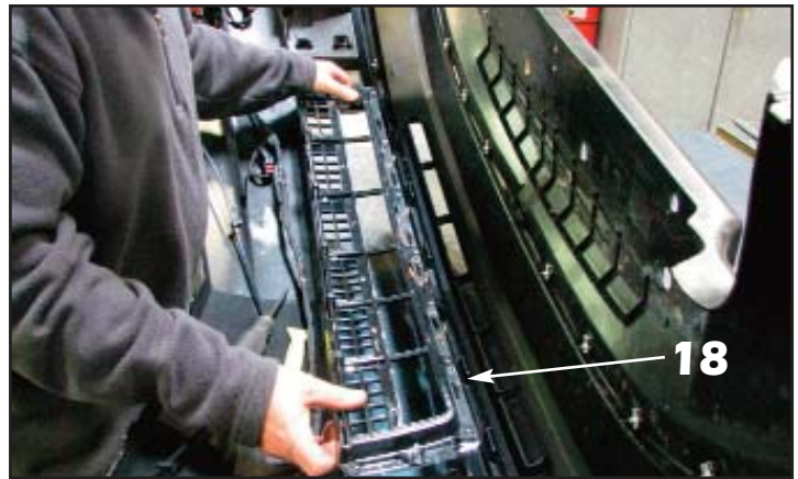
18. Once all the tabs have released, remove the lower factory grille from the bumper cover.
