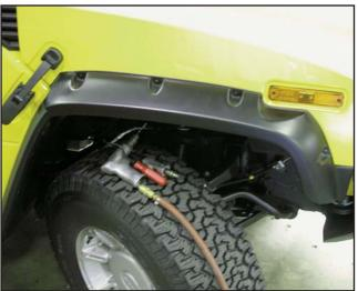
18. Align the E&G wheel arch flares over the factory wheel arch mouldings and reinstall the center push fasteners and factory mounting screws. Use a 9/64" drill bit to drill through the recessed areas and install the stainless steel hardware to finish. DO NOT OVER-TIGHTEN THE SCREWS I
