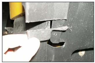
4. Trim off the lower section shown from the rear factory wheel mouldings (as shown).
