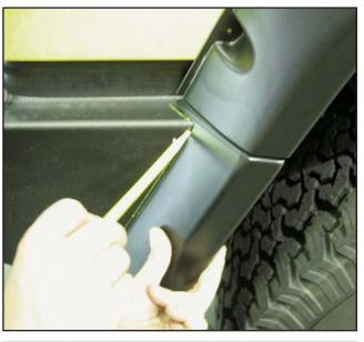
Align the splash guard sections to the rear flares and mark the bumper cover with a grease pencil. Remove the rear wheel flares for the following procedure.
