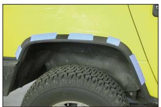
3. Remove the factory wheel arch moulding screws and use masking tape to align it back onto the while you align the E&G wheel arch flare. Keep most of the masking tape on the factory wheel arch, allowing only a 1/4" of tape to adhere to the body.
