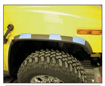
17. Tape the factory wheel arch moulding to the hood and remove the factory center push fastener and mounting screws (apply tape as out lined in step 3).
