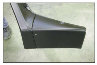
2. Once the rear extension is held in place with the 1" double faced tape, install two (2) 3/8" truss head screws to the bottom edge to secure it.
