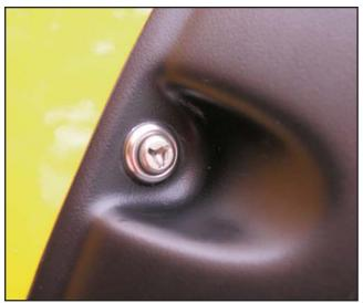
Install the rear wheel arch flares using the supplied stainless steel washers onto each tri-wing fastener and tighten. DO NOT OVER TIGHTEN OR YOU WILL STRIP OUT THE SCREW HOLESI
