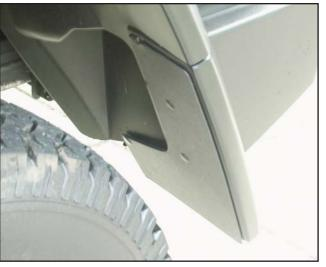
12. Install the supplied long push fasteners into the existing holes in the rear flare splash shields, rear flare splash guards and the factory rear bumper cover. Install a standard push fastener in the lower inside hole.
