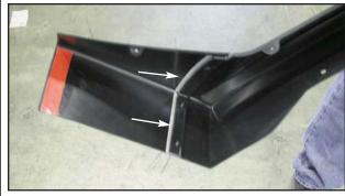
1. Attach the rear extension to the rear flares using the supplied double faced tape (where shown).
