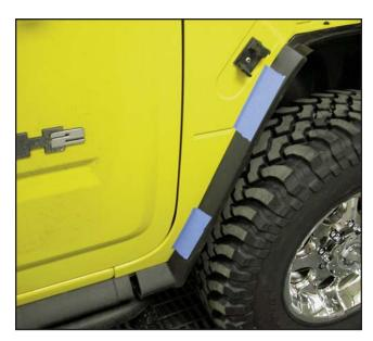
14. Align the factory wheel arch moulding back onto the cab and use masking tape to hold it in place (same procedure as rear off road flare).
