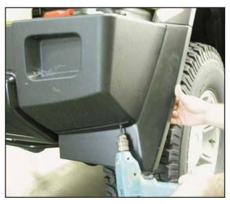
Align the rear splash guard sections. Drill (from underneath the vehicle) a 3/32" hole through the predrilled holes in the bottom rear edge of the E&G wheel splash guard section for 3/8" truss head screw installation.
