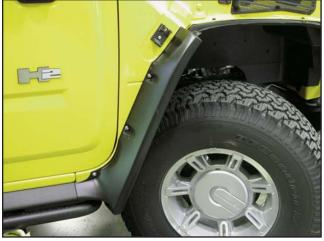
15. Align the E&G wheel arch flare over the factory wheel arch moulding and install it using the factory screws. Use a 9/64" drill to drill through the center of each mounting depression and install the supplied stainless steel fasteners. DO NOT OVERTIGHTEN THE SCREWS OR YOU WILL STRIP OUT THE MOUNTING HOLES I
