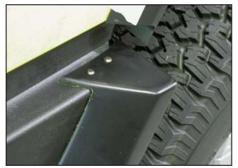
8. Once the rear flares have been removed, drill and install two (2) 3/4" truss head screws (where shown). Make sure the splash guards line up with the grease pencil marks. Blow out all holes drilled through the metal of the vehicle to remove metal shavings. Apply a qood quality sealer to each hole drilled to prevent future rust problems.
