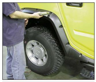
Align the E&G Classics fender flare over the taped on factory moulding and install them onto the vehicle using the factory screws (starting at top center). Use a 9/64" drill bit to drill through each recessed area in the flare for tamper-proof fastener installation.
