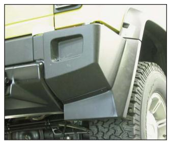
If the splashguard sections are slightly out of adjustment, simply move the inside edge forward or back, then drill and install a second (2nd) 3/8" truss head screw (see arrow).
