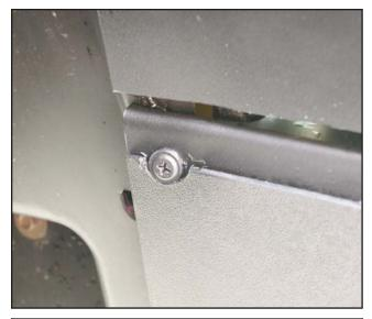
11. Align the rear splash shields into place, drill and install a 3/4" phillips truss head screw where shown at the top inside of the rear flare splash shield.
