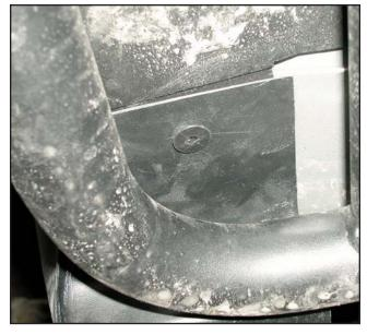
16. Once the factory screws are installed, align the bottom of the flare with the factory push fastener hole and reinstall the factory push fastener.
