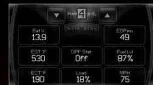
Monitors vehicle vitals by displaying up to 8 different parameters at a time
