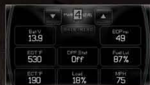
Monitors vehicle vitals by displaying up to 8 different parameters at a time on both the CS and CTS
