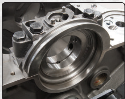
Block #450000 features a 2-piece rear main seal
