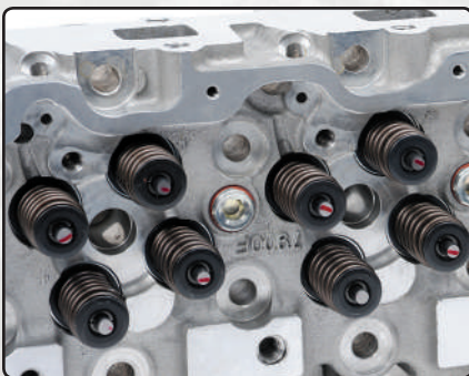
Injector cups are integrated into the castings for LB7 applications
