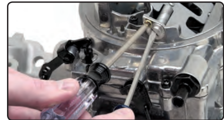
Our unique Qwik-Tune Secondary Air Valve can be easily adjusted with simple tools in seconds!
