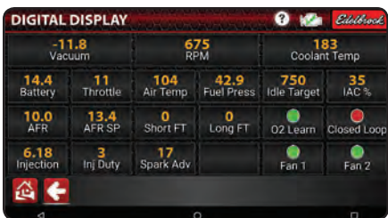
Pro-Flo 4 EFI system include an easy-to-use 7" Android touch screen tablet for setup and monitoring engine functions
