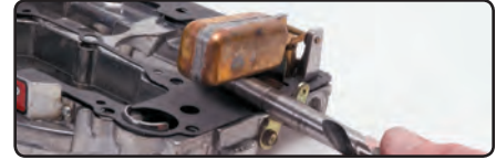
Checking float level with a 7/16" drill bit
