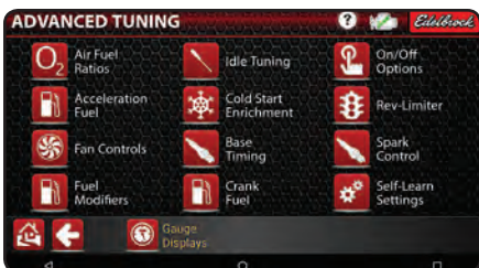
Pro-Flo 4 EFI system include an easy-to-use 7" Android touch screen tablet for setup and monitoring engine functions
