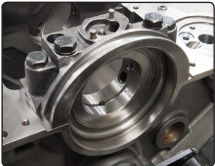
Block #450000 features a 2-piece rear main seal
