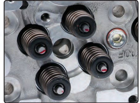
Injector cups are integrated into the castings for LB7 applications
