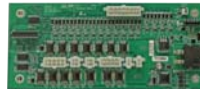
EZ2127CCXXX Driver board - for centrally controlled modules (Contact factory for programming requirements) Used with 21, 27 Series
