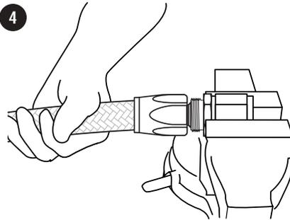
4. Holding the hose and not the socket, push the hose and the socket onto the nipple until the socket threads can be started on the cutter. Holding the hose and not the socket, start the threads and go as far as you can by hand. Depending on the size of the hose, some force may be necessary in this part of the operation.
