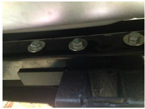
15) Tighten the 4 side bolts that are loosely inserted into the nut plates with a ratchet. Torque to 60 ft/lbs
