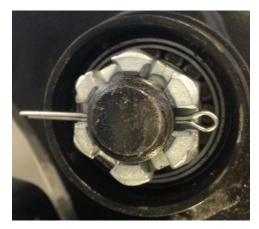
21)Bend the end of cotter pin to secure. Set the cap onto the whole assemble with the holes lined up that are highlighted below and then insert the small tapered head screw and tighten.
