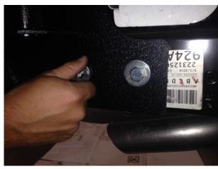
16) Ensure that the bumper is level. If it is not level repeat steps 12-15 making adjustments to level the bumper. NOTE: If the bumper is not level have a friend hold it level and tighten the side bolts first and then tighten the rear cross-member bolts. The bumper should be mounted
