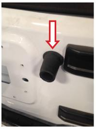
8) Next take the rubber donut and, using the *supplied hardware*, place it on the connector plate as shown in the drilled hole. UPDATE: Use the lower left hole.
