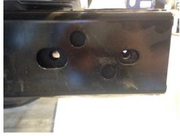
11) Next insert the 4 large 3"x 12mm through bolts through the frame rail with the threads facing the rear of the Jeep, make sure to put the washers onto the bolts as well. NOTE: You'll have to put the head of the bolt above the exhaust canister to get it into the hole.
