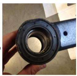
20) Carefully place the carrier back on the shaft with small bearing on top. Now add the fat washer before the castle nut. Tighten castle nut until it stops abruptly again and back off nut just far enough to get the cotter pin thru the hole in the shaft. NOTE: If you don't have enough room for cotter pin, that is a sign that you need to press the bearing race in a bit more. Simply put a little more torque on the castle nut and you will be able to press it in more.
