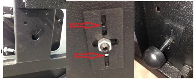
24) Make sure that the stopper lines up with the rubber donut as shown below. Adjust the inside nut to where the ball touches the donut when the carrier is just cracked open. Lock the ball in place with the outer nut. When the tire carrier is completely closed the ball will be pressed up against the factory rubber stopper. This will provide extra rigidity when there is a
