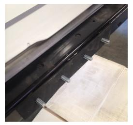
13) Have a friend or two lift the bumper with you and place the holes in the middle of the bumper on to the bolts sticking out of the rear of the frame. Install the nylon nuts on the 4 through bolts sticking out of the rear to hold the bumper to the frame. Next, install the short-
