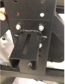
31) Place the final piece of the tire carrier into the slot shown below and use the two bolts provided to loosely attach it.
