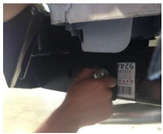
14) Next tighten the four center bolts in the rear cross-member first to allow the bumper to properly align itself. Torque to 60 ft/lbs.
