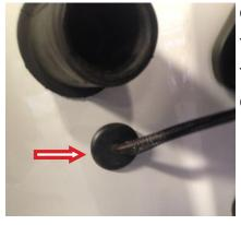
coming out easily, help the rubber fitting from the inside of the tailgate by pushing from the rear and pulling at an angle downward at the same time.
