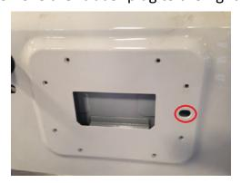
7) Remove the rubber stock tire stabilizer on the right from the tailgate. To remove, pull it out and rotating it at a slight angle to avoid damage. Leave the stabilizer, that is on the left
