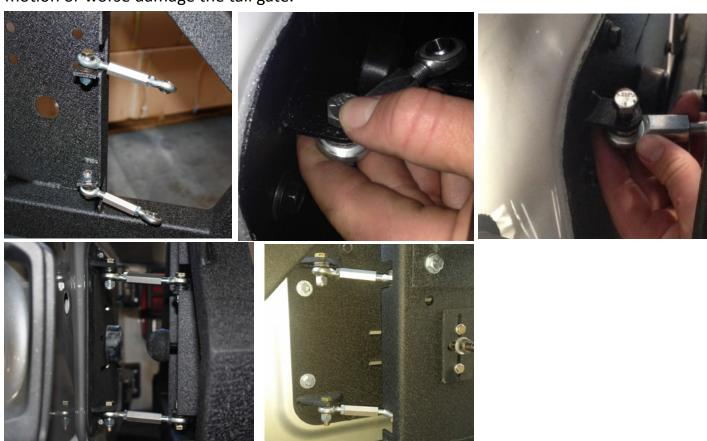
27) You can shorten or lengthen the heim joint by spinning the middle turn buckle until you have taken away any slack in the tire carrier. Any adjustments to the heims should be made when the door is closed. Tighten the jam nut on the turn buckle when you are finished setting the length, this will ensure it wont back off when your driving.
