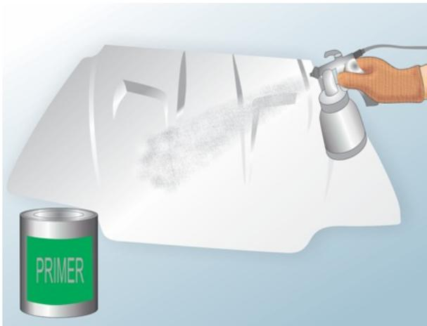
**Apply primer to the fiberglass.** Once the component has been sanded with coarse-grit sandpaper, apply the primer and allow it to set. Avoid using etching primer, as it won't adhere well to fiberglass.
