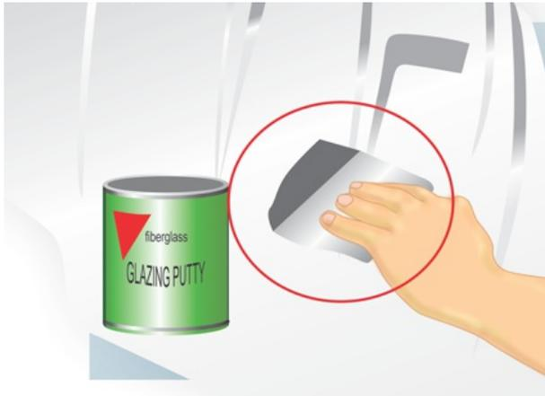
**Fill any low spots in the fiberglass.** To raise the profile of low spots in the surface, use a fiberglass glazing putty. Work the putty into the low spot, and then sand it away until the area is flush with the rest of the surface.
