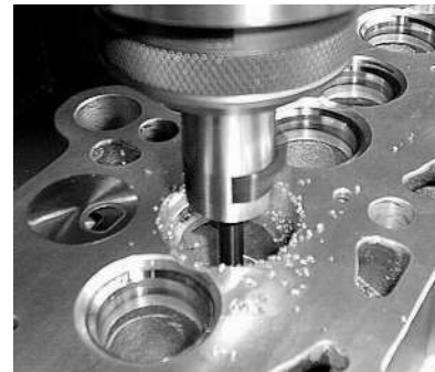
Picture 5 - Cutting the counter bore
