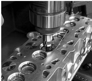
Picture 3 - Cutting valve seat inserts
