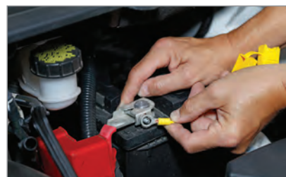
3. Route T-One® Connector to the tail light harness.
