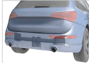
Euro Hitch installed with receiver box removed
