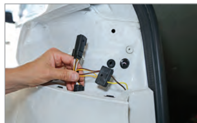
3. Route T-One® Connector to the tail light harness.
