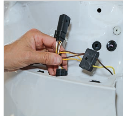
3. Route T-One® Connector to the tail light harness.
