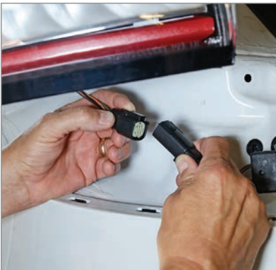
4. Plug the tail light into the T-One® connector.
