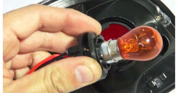
7. In comparison to your stock tail lights, LED lights function at a lower wattage and include a resistor that regulates the current passing to the lamps. In some cases, this box can be internal, but generally it is external and connected via a plastic plug. By the way, the latter type should be mounted (they usually come with a double-sided tape on the backs) where it will be far from moisture and heat.
