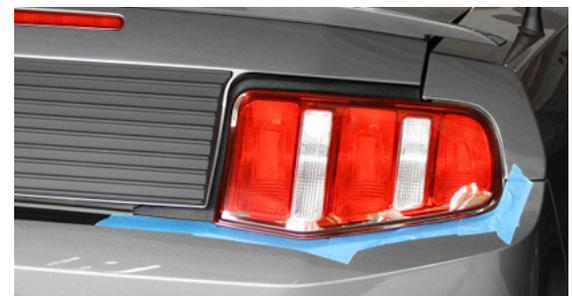
4. To carefully remove your stock lights, open your tailgate or trunk lid to access the back panel of your tail lights. Unscrew your worn out tail lamps from the front with the help of a Phillips screwdriver or undo of the bolts is released, your old lights may fall instantly. For this reason, it is better to lightly keep the lights in place with your free hand while you unscrew or unbolt them.
