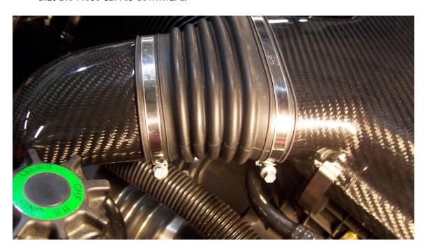
21. Locate the **D762-0115 Carbon Intake Tube** and one **#48Z (80-100) Hose Clamp**. Fit the clamp onto the Airbox Hose as shown previously and install the Tube down into the space below the headlights and into the Hose. At this point you may be able to tell if there is sufficient clearance between the relocated horn and the Intake Tube. Readjust the horn if necessary. Tighten the hose clamp with the Intake Tube rotated so it has the most "wiggle room" at its lower end.
