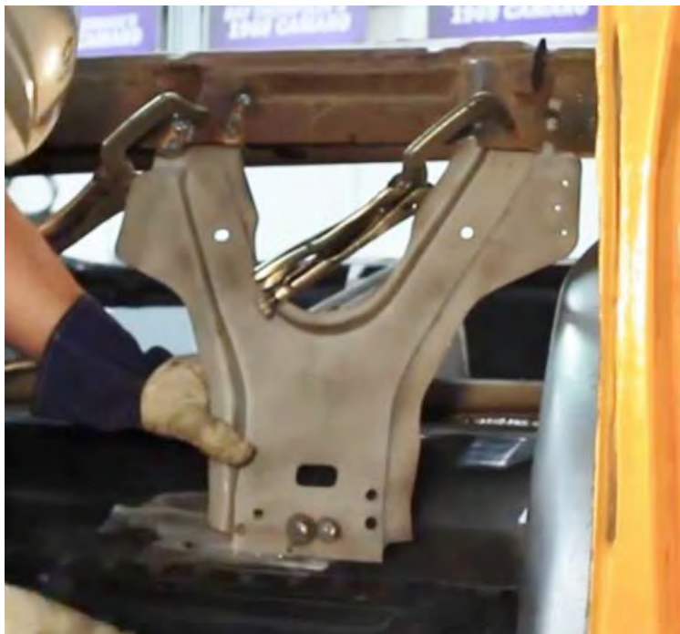
Figure 45 - Weld in Package Tray Reinforcements
