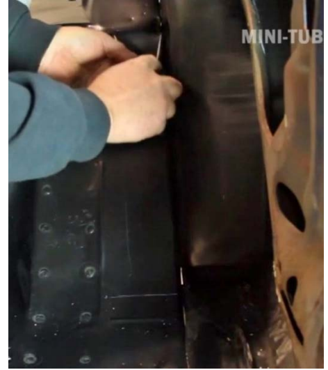
Figure 5 – Set Dividers and Transfer a 2-3/4" Scribe Line
