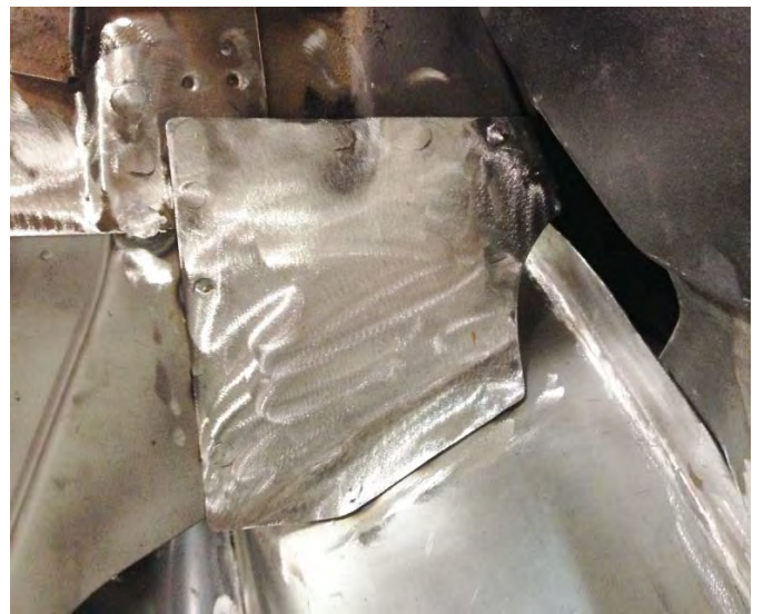
Figure 47 - Weld in Rear Seat Bracket Closeout
