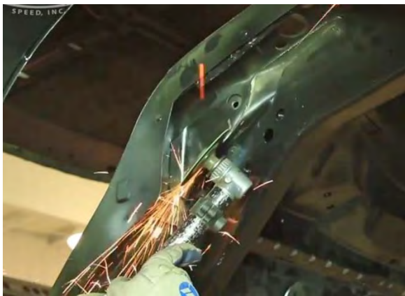
Figure 22 - Cutting the Frameraill Reinforcement
