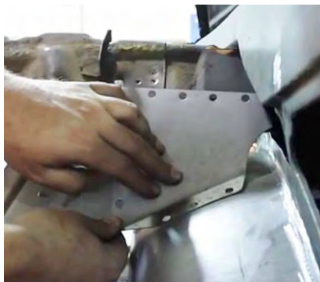
Figure 46 - Rear Seat Bracket Closeout
