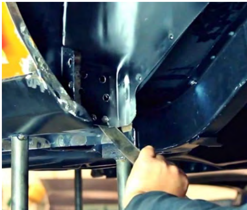
Figure 14 – Separate the Inner Wheel Tub from the Rocker
