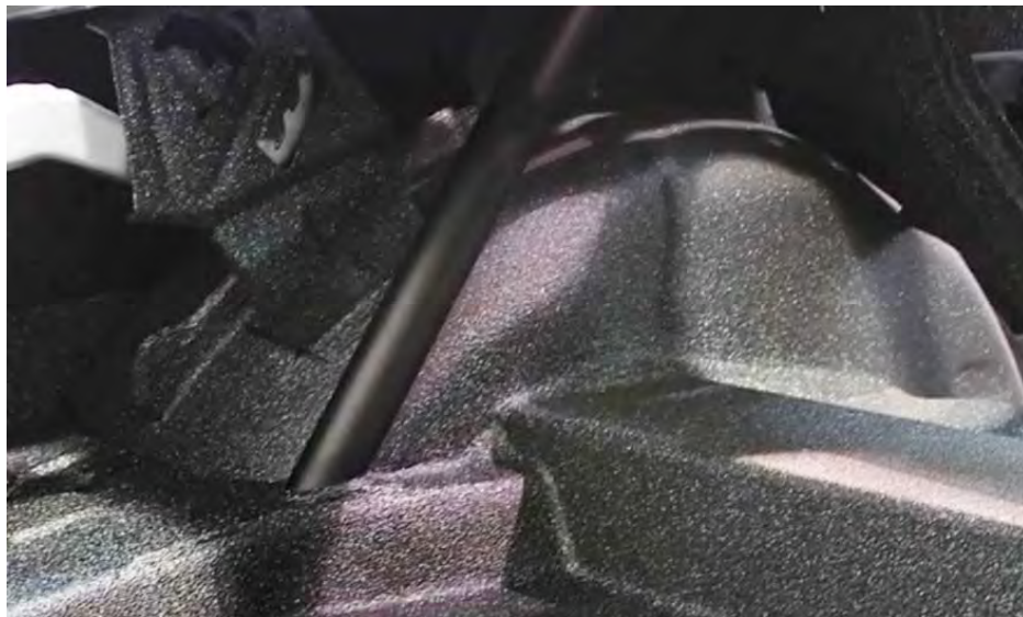
Figure 48 - DSE Mini-Tubs Completed
