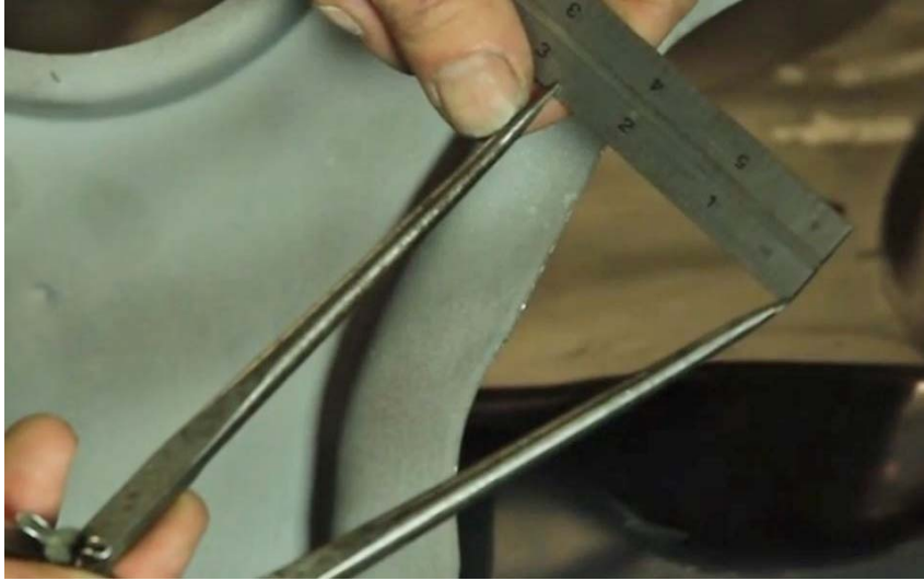
Figure 5 – Set Dividers and Transfer a 2-3/4" Scribe Line
