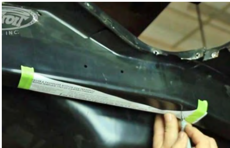
Figure 24 - Scribe Cut Line onto the Bottom Frameraill
