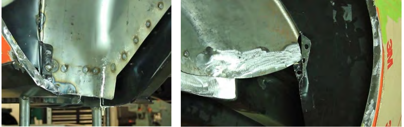
Figure 40 - Weld Outer Wheel Tub Flanges
