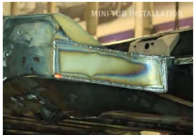
Figure 31 - Install Framerrail Closeout
