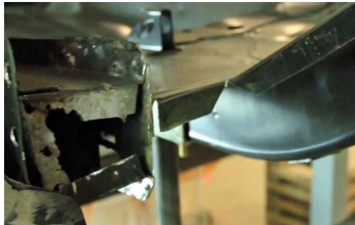
Figure 28 - Trim Rocker and Bend Fold Lines
