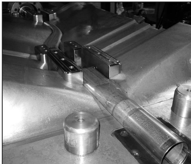
The frameraill is set in place for hydroforming
