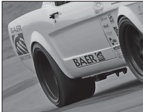
**Tech Tip:** Although backspacing can vary, Detroit Speed recommends at least 5.500" for rear caliper clearance.
