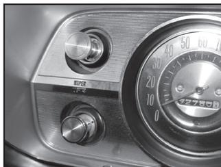
Matching wiper kit knob installed in a 1965 Chevelle
