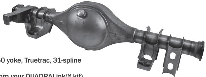
9" rear axle with QUADRALink™ bracketry installed
