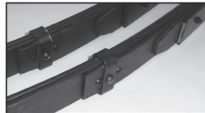
Tapered leaf springs with anti-friction pads
