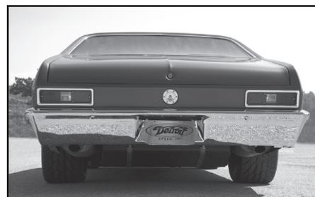
Mini-Tub Kit with 3" drop is installed on this 1972 X-Body
