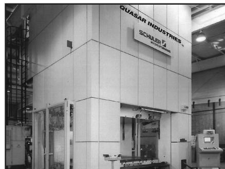
The large hydraulic press where the frameraills are made
